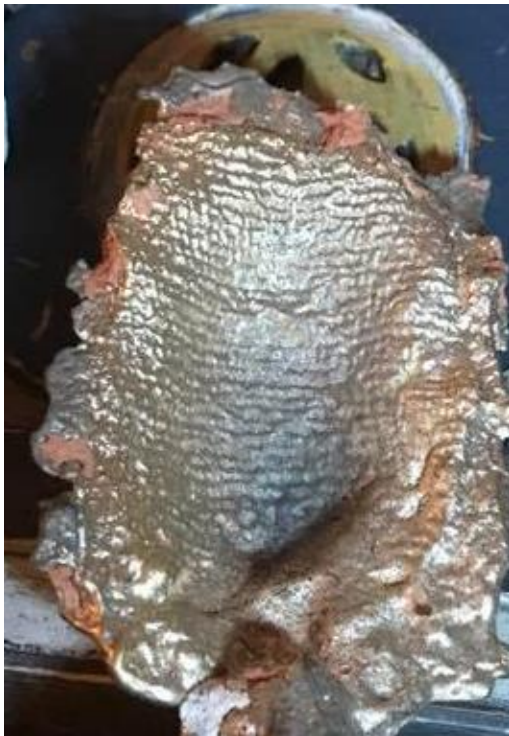
Fig. 16: Back of cast #1: while the casting was far too thick, the vaporized wool cloth is visible, similar to Smith's findings, and that of extant period pieces.
