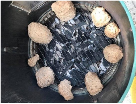
Fig 1: Initial heating of the moulds. More charcoal will be added around the moulds after an hour.
