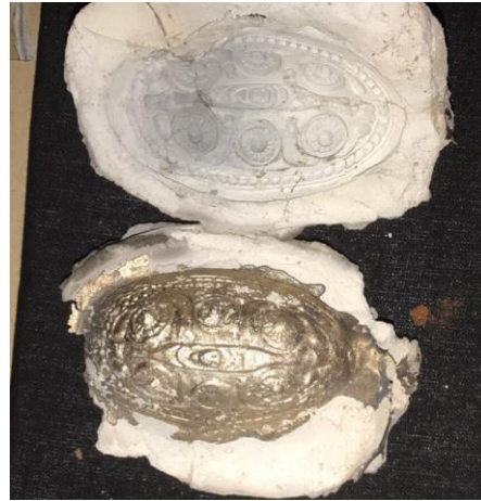
Fig 15: A completed cast. Note the low level of detail. This is somewhat common with direct-matrix casts.
