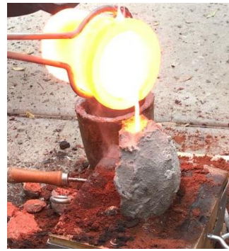
Fig 2: Taking the melt. If the mould is hot enough, the melt should pour in safely.
