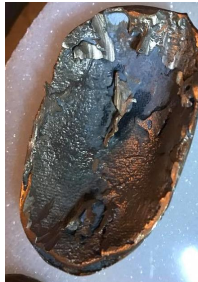
Fig 17: Cast #2: a more successful cast, though the pin-mounds did not fully cast. The wool markings are still present.
